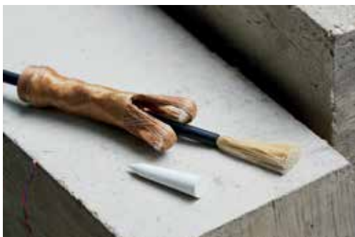
Fully composite anchors developed for aramid ropes
